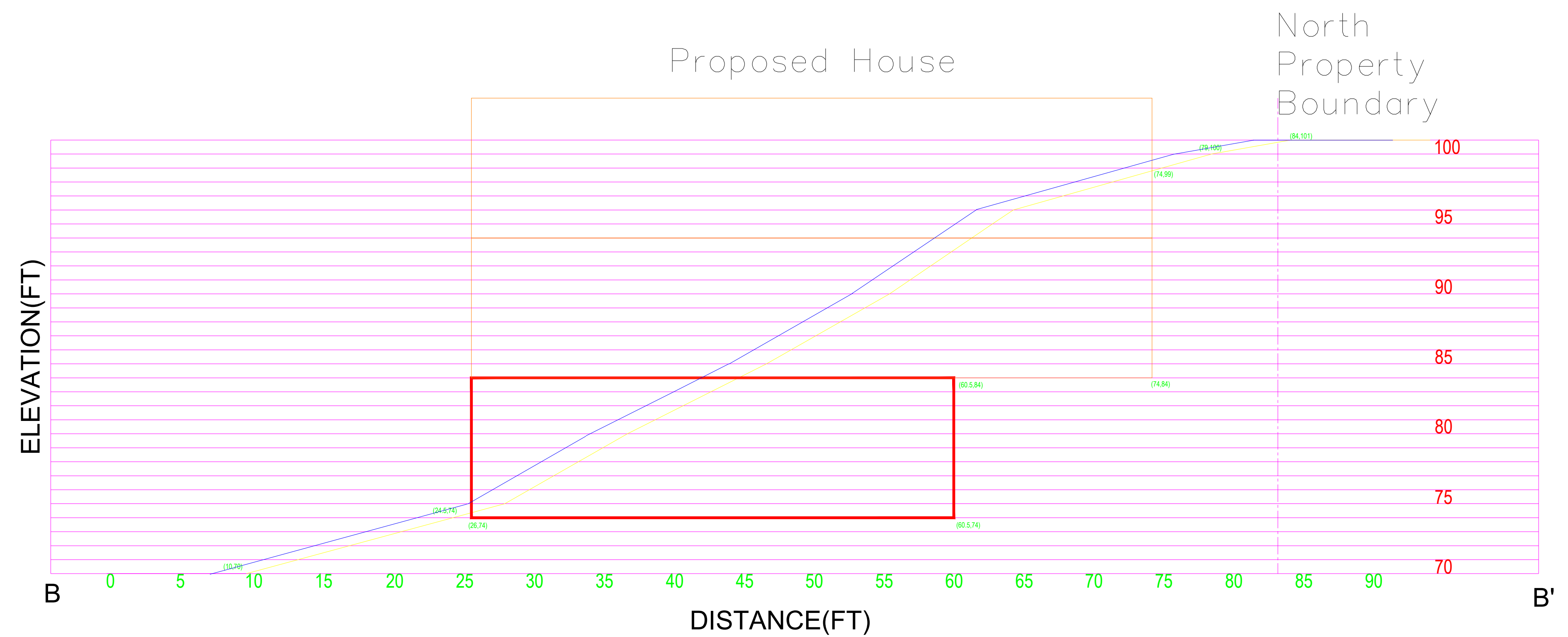
SOUTHWEST FACING SLOPE CROSS SECTION B-B'
